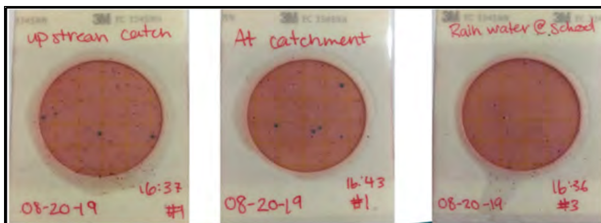
Figure 7. Water quality test results illustrate the presence of E. coli and coliforms in the three water samples [1]
